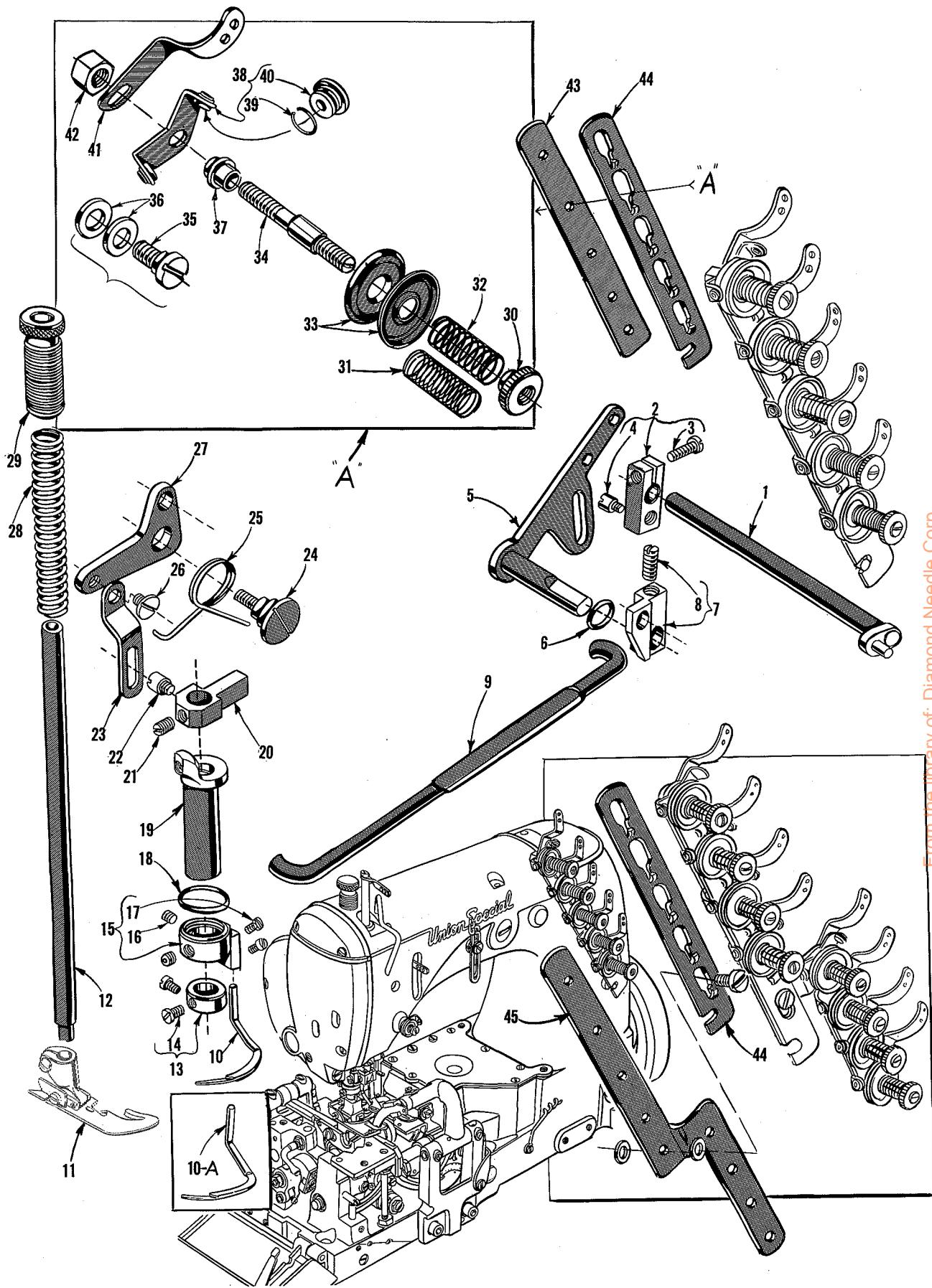
**THREAD TENSION, LIFTER LEVER PARTS AND SPREADER HOLDING PARTS**
