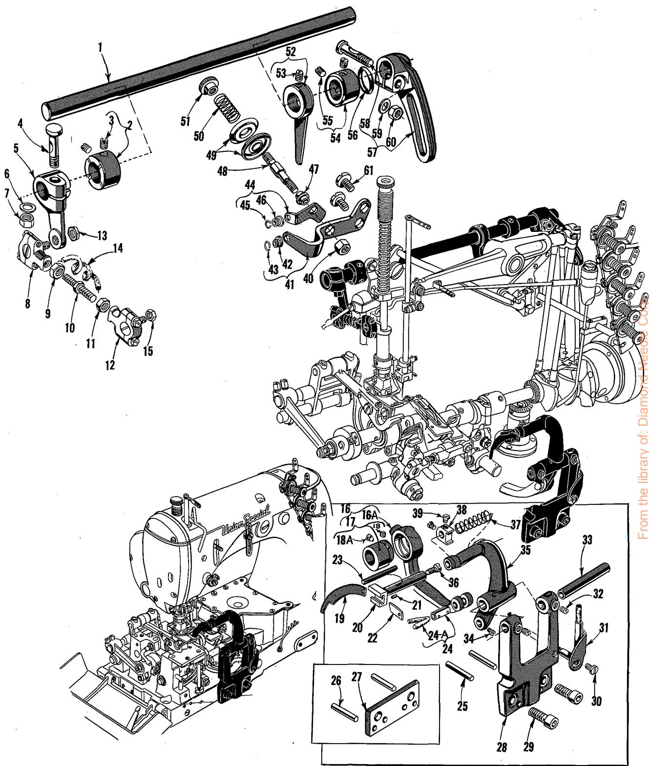
UPPER KNIFE AND SPREADER DRIVE MECHANISM
