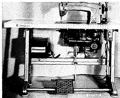
**AMCO ELECTRONIC NEEDLE POSITIONERS** eliminate the necessity of reaching for the hand-wheel to move the needle up or down . . . this allows the operator to keep both hands on the work, insuring better control, uniform quality and increased production.
