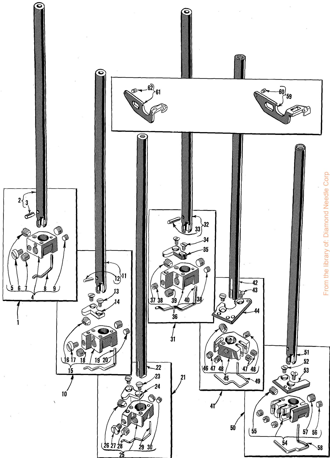
NEEDLE BARS, NEEDLE HOLDERS AND NEEDLE GUARDS
