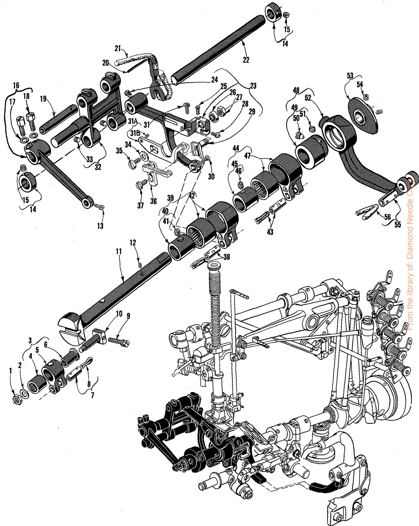
MAIN SHAFT AND FEED MECHANISM
